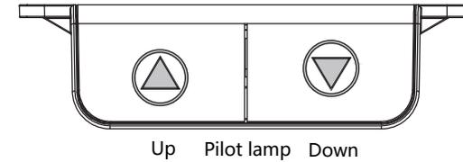
When using it for the first time, please press the "▼" down running key, when it runs to the bottom, the buzzer will make a sound of "di", and it can run up or down normally.
